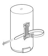
Lead the end of the pole mounting strap through the back of the Deco.
