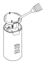
Loosen the screws to detach the waterproof cover of the Deco with a Phillips screwdriver.
