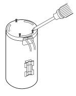
Replace the waterproof cover, leading the cable(s) through the slot(s) of the waterproof rubber.
