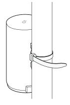
Position the Deco and wrap the pole mounting strap around the pole.
